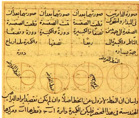
Fig. 10.0.4. Tūsī's diagram of the couple, showing the oscillation of a given point along the diameter of the big circle. After Tūsī couple from Vat. Arabic ms 319 , commons.wikimedia.org, Creative Commons Licence
