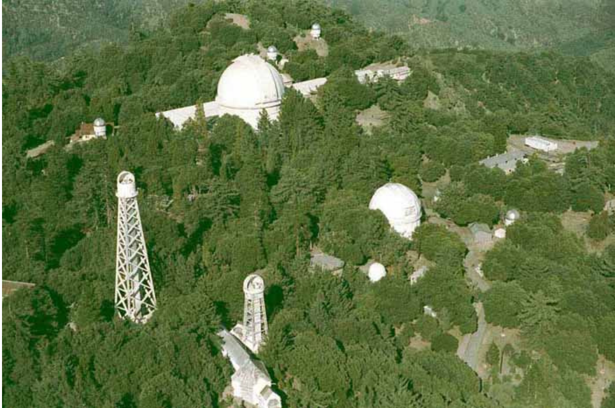
Fig. 12.4.1. Aerial view of the Mount Wilson Observatory: In the lower-left are the 150ft and 60ft solar tower telescopes; in front is the horizontal Snow solar telescope. The domes of the 60-in and the 100-in Hooker telescope are visible behind. Photograph © Norm Vargas ( http://www.mwoa.org/ ).
